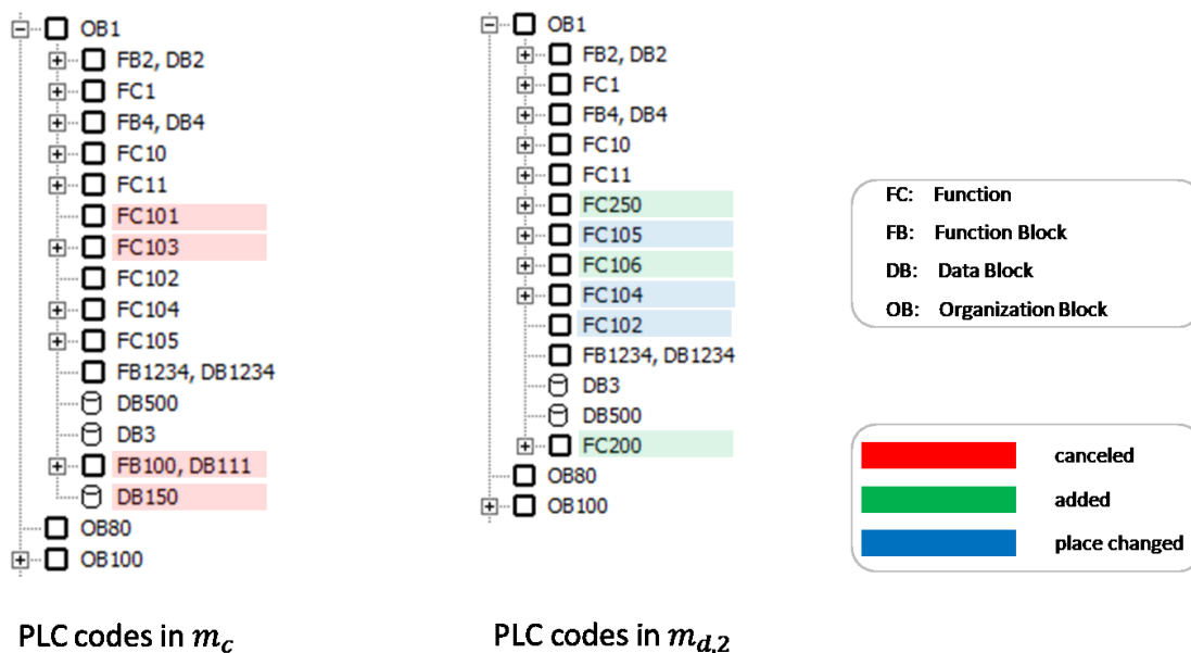
Figure 111: Comparing software codes in control system between m_c and m_{d,2}
